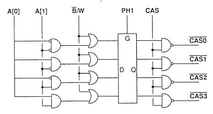
CASO drives the DRAM bank which is connected to D[0:7], CASI drives the bank connected to D[8:15], and so on. This has the added advantage of reducing the load on each column strobe driver, which improves the precision of this time critical signal.
